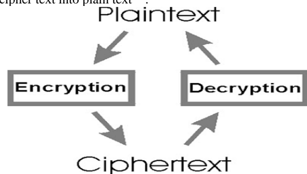
Figure 1: Conversion of plain text to cipher text and vice versa
